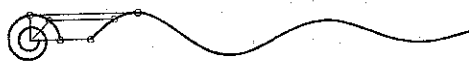
A damped oscillator in state space form. Left: At each time step the state vector, s_t , rotates by \omega and its length becomes shorter. Right: The actual waveform is a one dimensional projection from the two dimensional state vector.
